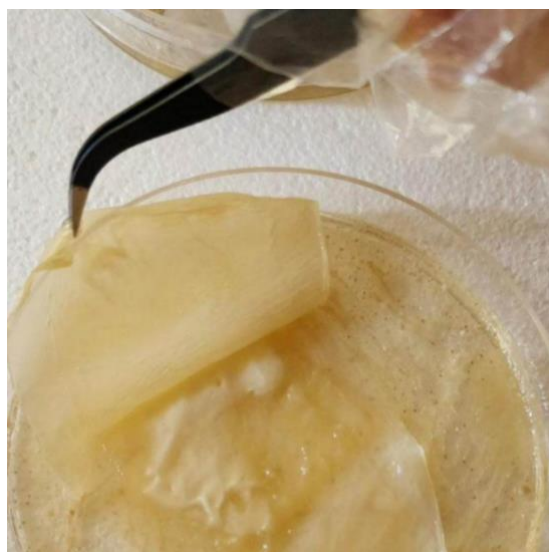
Figure 1. Laboratory technique for natural dye application using sterile tweezers to handle BC film in turmeric solution, demonstrating a controlled dyeing process at room temperature.
